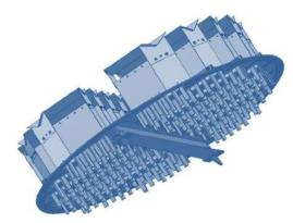
A mixed feed that flashes when it enters the column between beds can lead to maldistribution. In this instance, there may be a requirement for a complex inlet distributor design that produces both, an even composition and flow rate at each point in the column cross section.
