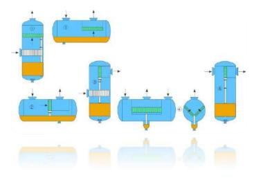
As the hydrocarbon gas/oil/water mixture is extracted from below the sea bed, the mixture is fed into a production separator vessel on the offshore platform.
