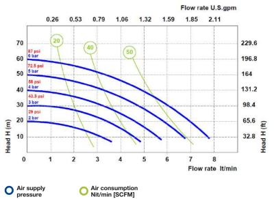
The curves and performance values refer to pumps with submerged suction and a free delivery outlet with water at 20°C. These data may vary according to the construction materials and hydraulic conditions.
